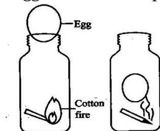
A glass bottle is taken, inside the bottle, put some pieces of cotton with fire. Then place a boiled egg, the temperature inside the bottle increases from the fire rising the pressure.
